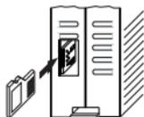
Inserting the MicroSD or the microSDHC, into the side slot. Max 32 GB.
