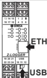
The module has a RJ45 socket on frontal panel.
