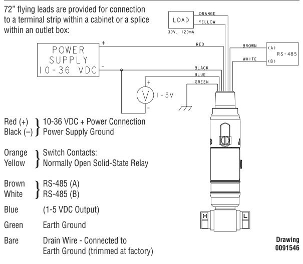
NOTE: An external ground screw is included for additional earth ground connection.
