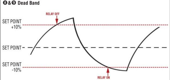
The diagram above depicts an adjustable dead band. Dead band is the range through which an input can be varied without initiating an observable response. Dead band is usually expressed in percent of span.
