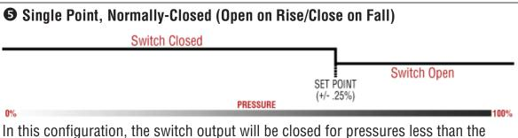
In this configuration, the switch output will be closed for pressures less than the selected setpoint. The switch output would then be open for pressures greater than the setpoint.
