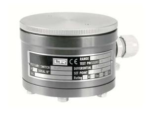
These diaphragm pressure switches are IP 55, and only suitable for applications where IP 55 execution is permitted. The sensing element is a metallic diaphragm and acts directly on the microswitch through a self-centering pivot. The simplicity of the design, without levers, cams or similar mechanism, gives the unit an exceptionally long working life.
