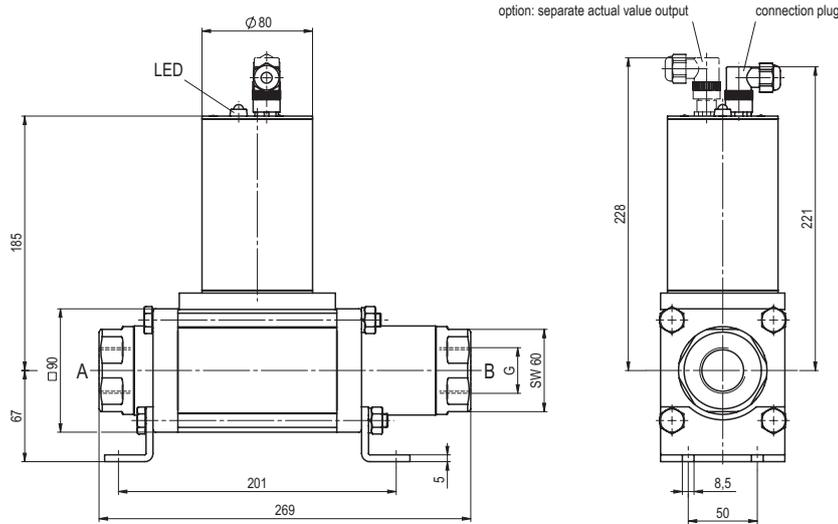
Mounting orientation can be vertical or horizontal, actuator cannot be installed facing down
