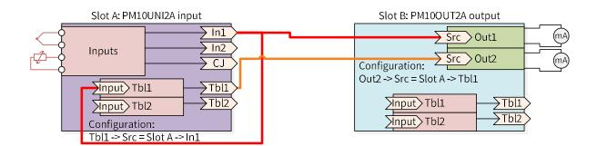
When a block uses a register of the same card as its input (like slot A Tbl1 uses slot A In1 in the example above), there are two ways to refer to the register:
