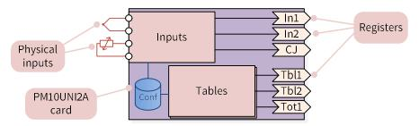
If you plug an analog output card in a PM10 device, the output will not work as it doesn't know what it should do. In addition to selecting the traditional signal type and the scaling, you must define, what the output is following or representing – the first analog input, the second, or something very different. The same applies for any kind of output, including the display – the source register must be explicitly configured.
