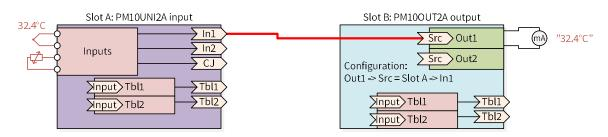
A register can be used by many blocks, and in the same or different card. As an example, we want to have another analog output that is linearized with a table:
