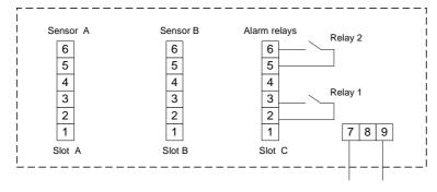
Outputcard or relaycard is installed on slot C.
