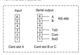
By serial signal RS-485 last unit must be terminated by 110 ohm resistor. you can make termination at terminal connectors or by connecting jumper J1 to ON-position.
