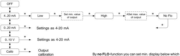
By **no FLO**-function you can set min. display below which output drops to zero (or to 4 mA). This method fastens updating of output when incoming pulses have stopped.
