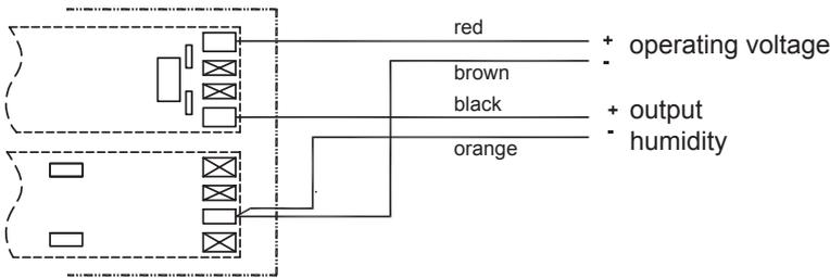
**Pin assignments sensors with connecting head IR..., IT...**
