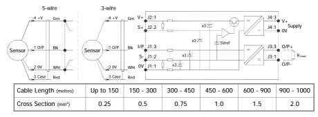
The table above shows recommended conductor sizes with respect to cable length for both three and five wire connections, based on copper conductors. Three wire connections will introduce a gain reduction of 5% and a ±1% temperature dependence of gain over the range -40°C to +80°C for the cable temperature. (i.e. about -150 ppm/°C for the maximum lengths shown and less pro rata for shorter lengths.)
