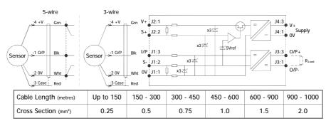
The table above shows recommended conductor sizes with respect to cable length for both three and five wire connections, based on copper conductors. Three wire connections will introduce a gain reduction of 5% and a  $\pm 1\%$  temperature dependence of gain over the range -40°C to  $\pm 80$ °C for the cable temperature. (i.e. about  $\pm 150$  ppm/°C for the maximum lengths shown and less pro rata for shorter lengths.)
