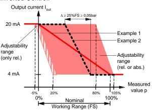
Programmable Damping of the Current Output
