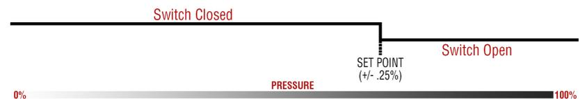
In this configuration, the switch output will be closed for pressures less than the selected setpoint. The switch output would then be open for pressures greater than the setpoint.
