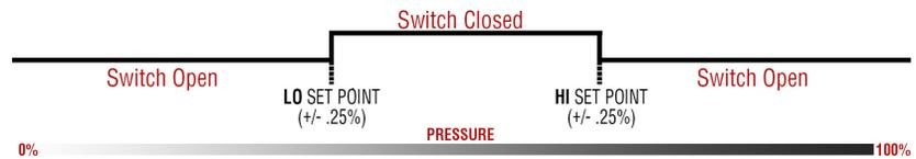
In this configuration, the switch output will be closed when the process pressure is within a user selectable range and open when the pressure is outside of these boundaries. This is designed for applications where there is a known acceptable operating pressure range.
