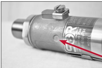
The 815LT can be easily configured externally with a magnet. Simply place a magnet to the targets located on the housing for 3 seconds and set the zero and span.
