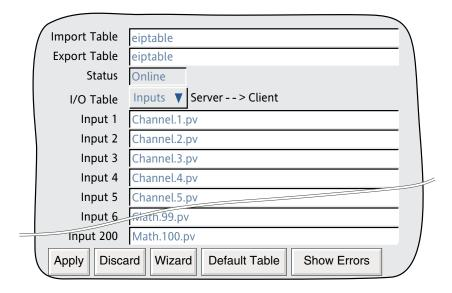
Figure 4.3.21a Ethernet/IP option configuration (large frame unit)
