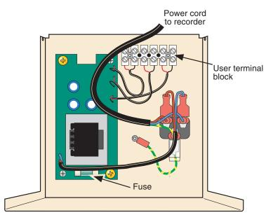
Figure 11.2.2c Fuse and User terminal block locations.
