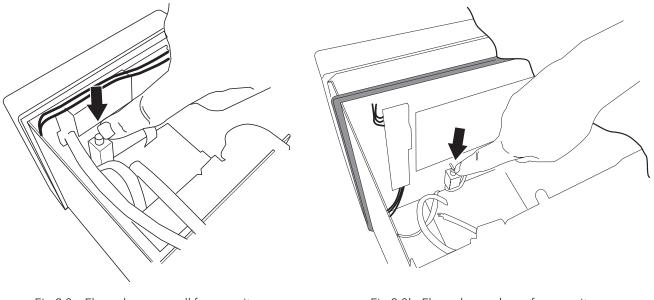
Fig 2.3a Flap release - small frame units
