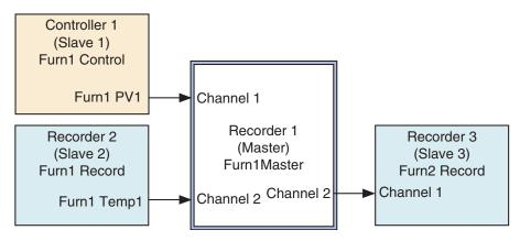
Figure 4.3.16j Required setup
