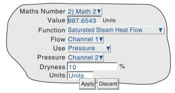
Figure 4.3.11j Typical Saturated Steam Heat Flow configuration page
