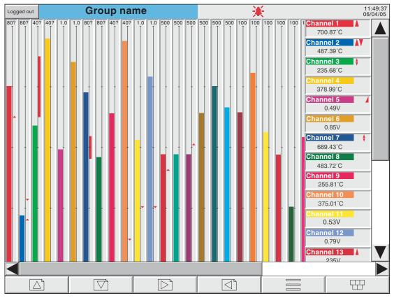
Figure 3.4.4b Vertical bargraph display (more than 6 channels)
