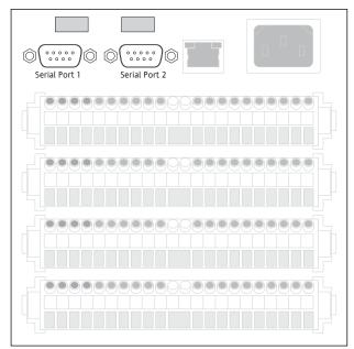
Figure 12.2.1a Serial port locations (small frame)
