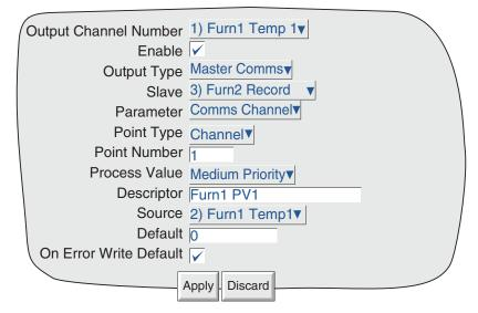
Figure 4.3.16m Master Output 1 setup example
