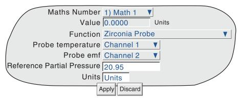
Figure 4.3.11r Zirconia probe function configuration menu
