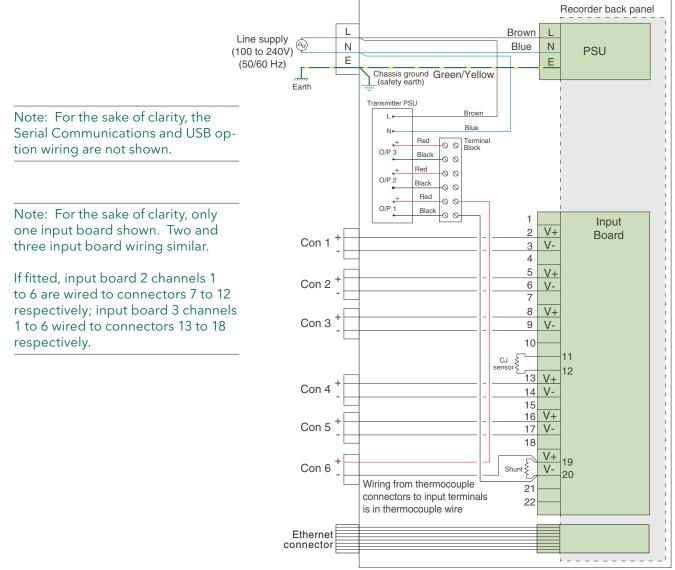
Figure 13.3.2c Internal wiring details
