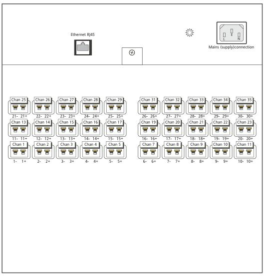
Figure 14.1.2b Rear panel connector layout
