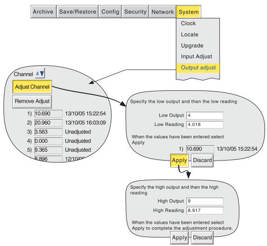
Figure 9.4.1 Typical output adjust pages
