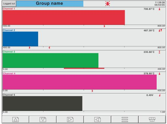
Figure 3.4.5a Horizontal bargraph display (single column example)
