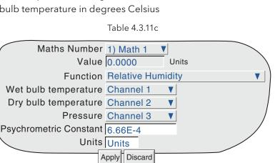
Figure 4.3.11q Relative humidity configuration menu
