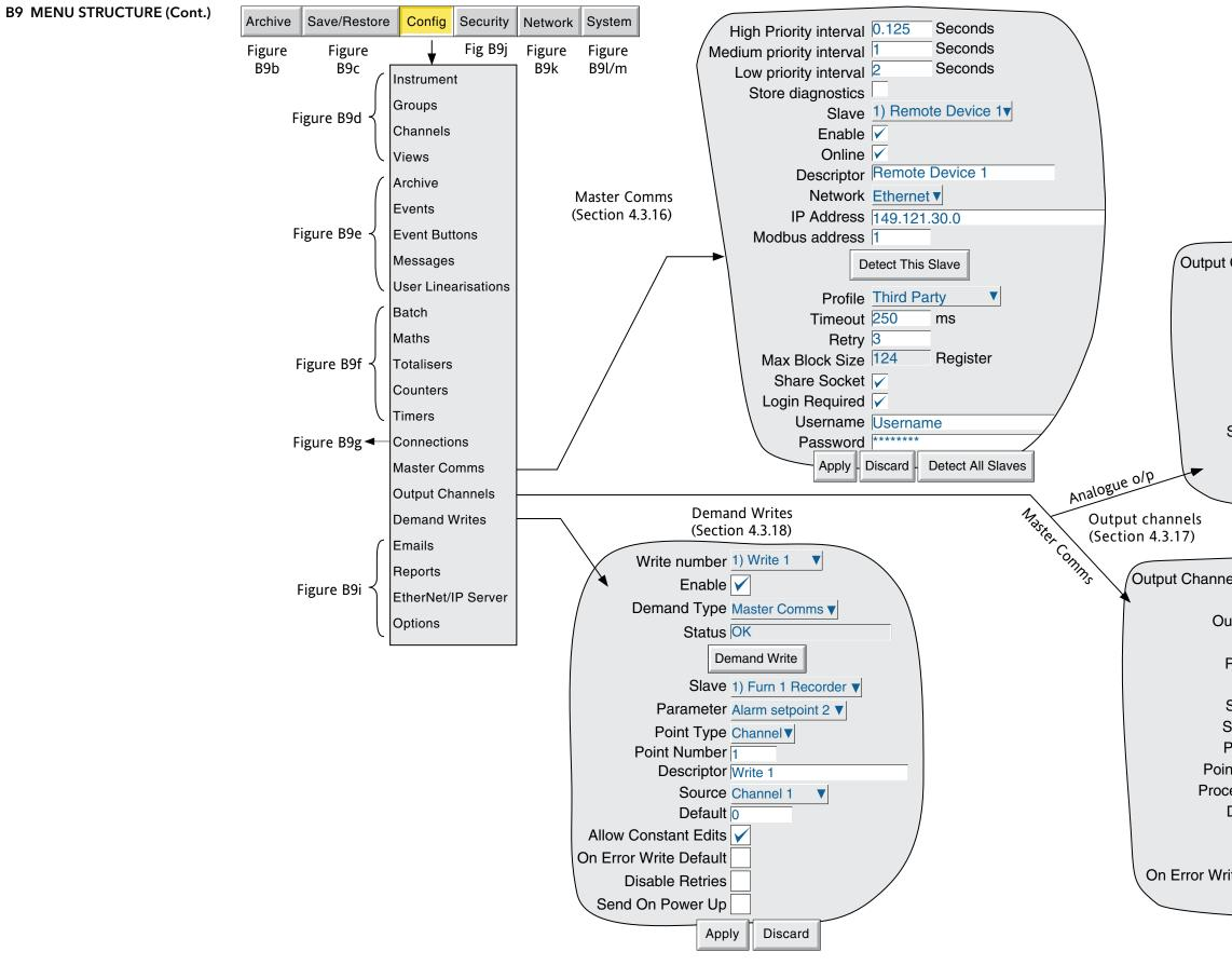
Figure B9h Config menu structure (sheet 5)
