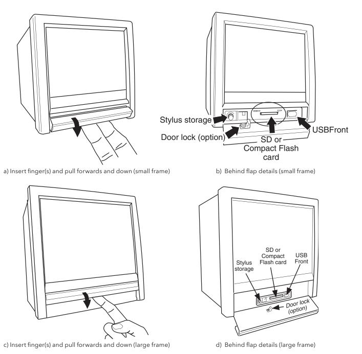
Figure 2.3 Access flap detail
