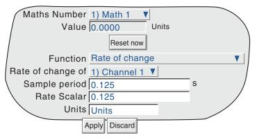
Figure 4.3.11n Rate of change configuration menu
