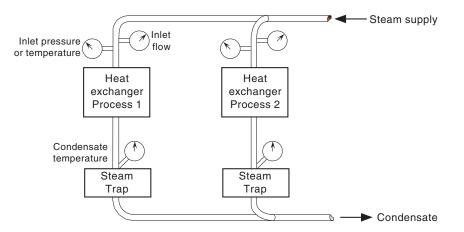
Figure 4.3.11k Measurement transducer - typical locations
