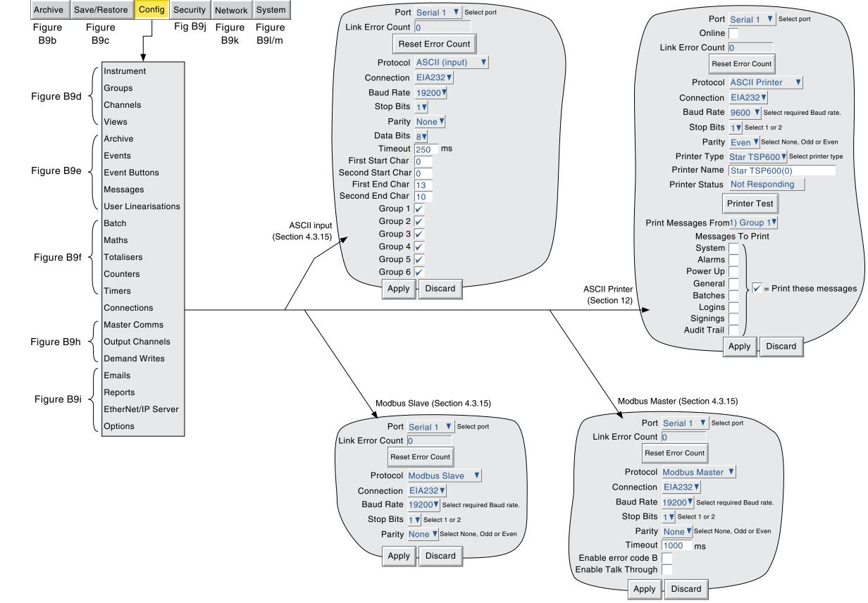
Figure B9g Config menu structure (sheet 4)
