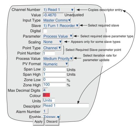
Figure 4.3.16e Channel configuration page - Typical Recorder
