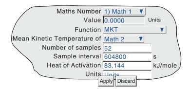
Figure 4.3.11g MKT function parameters
