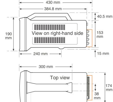
Figure 13 Portable case dimensions
