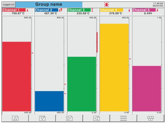
Figure 3.4.4a Vertical bargraph display (1 to 6 channels)
