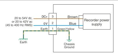
Figure 13.5a Internal wiring for low voltage options
