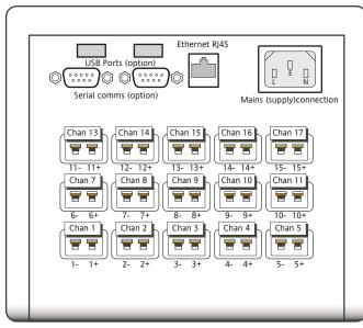
Figure 13.6.2a Rear panel connector layout
