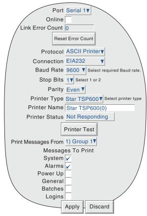
Figure 12.3.1a Serial communications configuration menu
