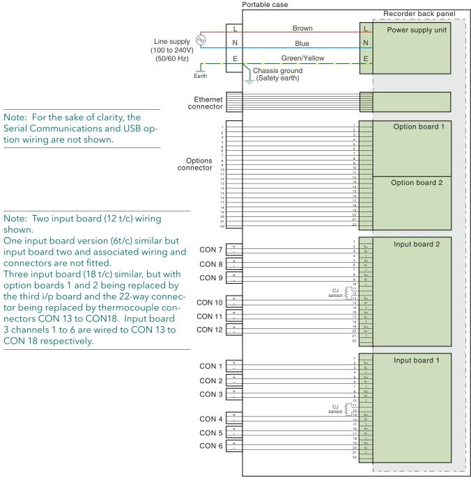
Figure 13.4.2c Internal wiring
