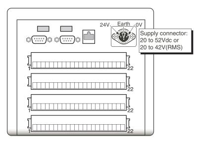
Figure 13.5b Low supply voltage connector details
