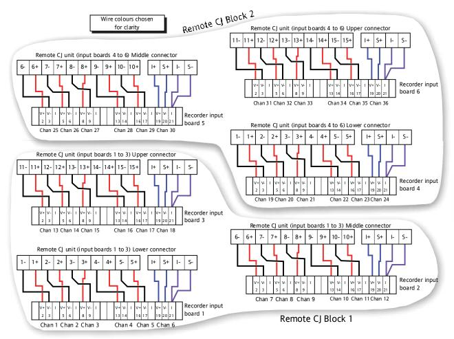
Figure 14.2.2c Wiring details
