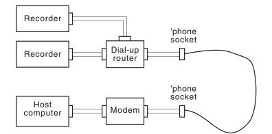
Figure 6.2.2 Remote connection example
