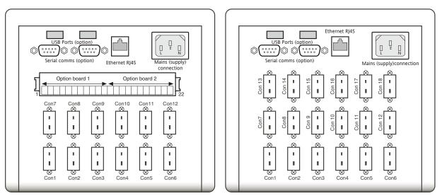
Figure 13.4.2a Rear panel connector locations (typical)
