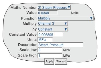
Figure 4.3.11i PSI to MPa conversion example
