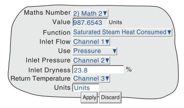
Figure 4.3.111 Typical Saturated Steam Heat Flow configuration page
