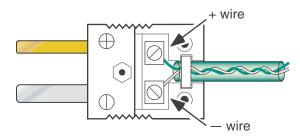
Figure 14.1.2a Connector detail (typical)
