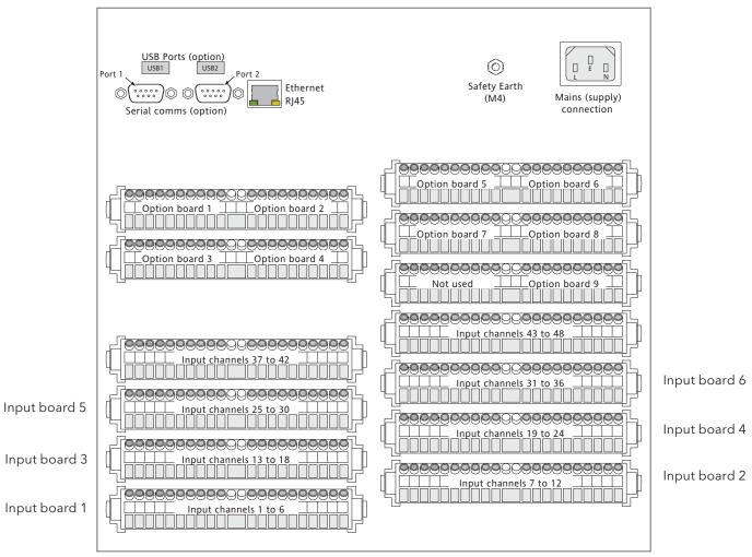
Figure 14.2.2c Connector locations (recorder)
