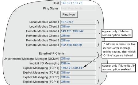
Figure 4.6.7 Ethernet Diagnostics display
