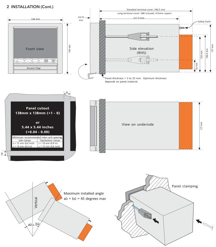
Figure 2.1a Mechanical installation details - small frame unit
