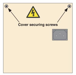
Figure 11.2.2a Retaining screw locations
