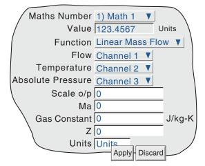
Figure 4.3.11d Linear mass flow menu
