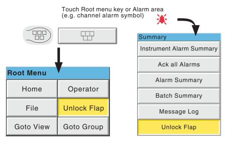
Figure 2.4.1a Unlock Flap key locations
