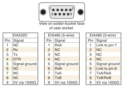
Figure 2.2.1d (Cont.) Option wiring sheet 2 (Serial communications)
