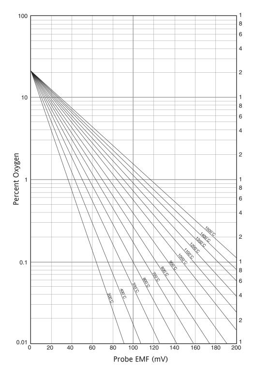
Figure 4.3.11s Probe emf versus temperature
