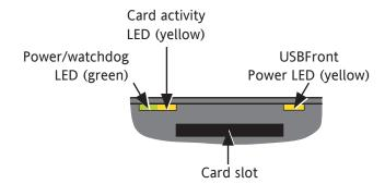
Figure 2.3.2c indicating LEDs (SD card - Compact Flash card similar)
