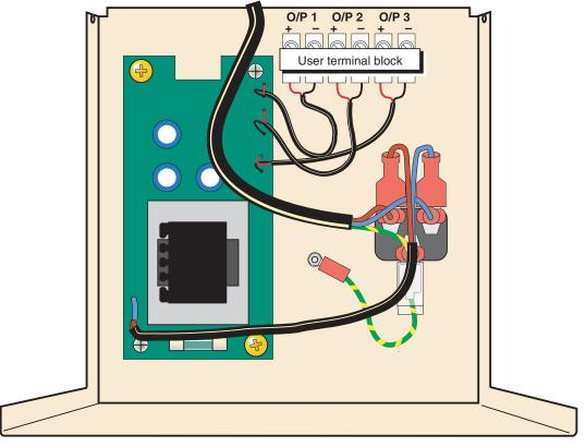
Figure 11.2.3a Terminal block wiring
