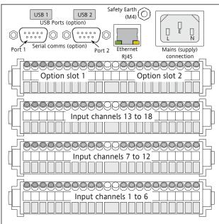
Figure 2.2.1a Connector locations - small frame units
