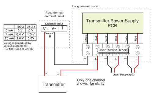
R (minimum spec) = 1.4W,  $\pm$  1%. 100 $\Omega$  or 250 $\Omega$  as required (see table)
