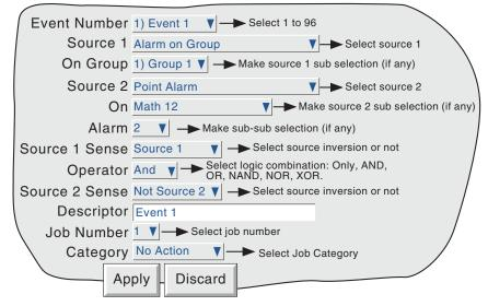
Figure 4.3.6 Event configuration menu layout (typical)
