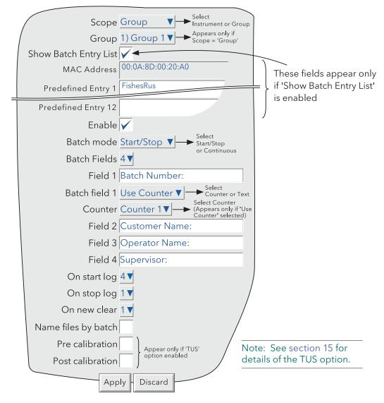
Figure 4.3.10a Batch configuration menu
