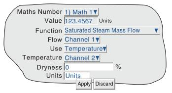
Figure 4.3.11h Typical Saturated Steam Mass Flow configuration page
