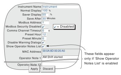
Figure 4.3.1 Instrument Configuration menu
