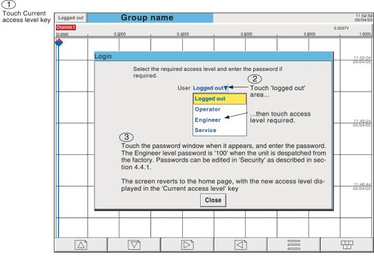
Figure 3.3.1a Access to configuration
