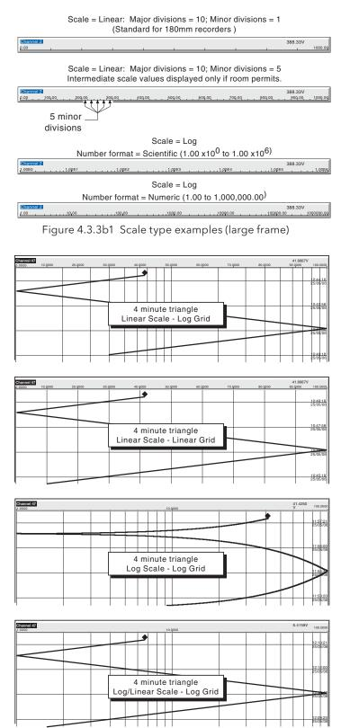
Figure 4.3.3b2 Trace examples for different scale types (large frame)
