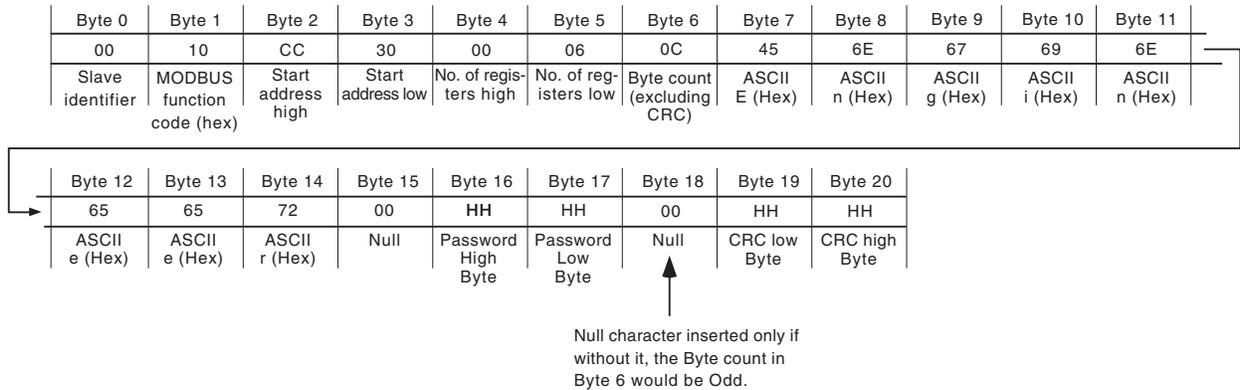
Figure 8.2.4b Login Request using a serial transmission line.
