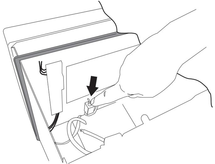
Fig 2.3b Flap release - large frame units
