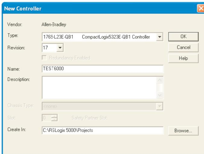
Figure 4.3.21g New Controller window
