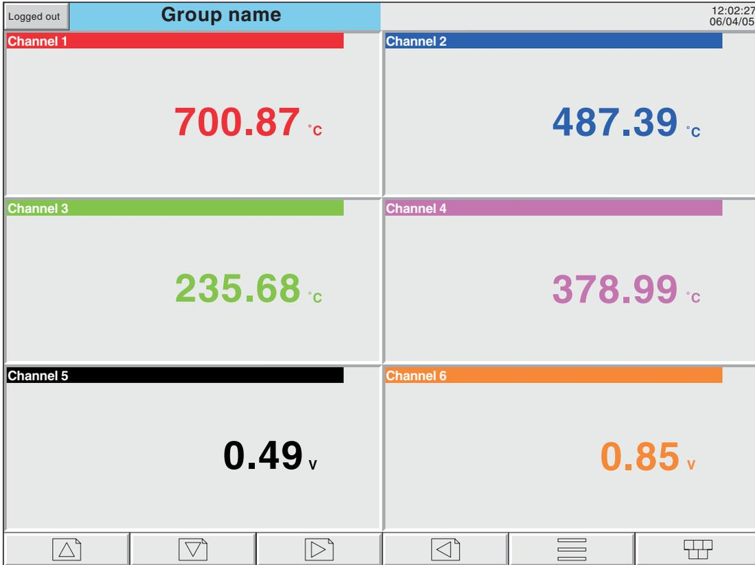
Figure 3.4.6b Numeric display mode example (6 channels)
