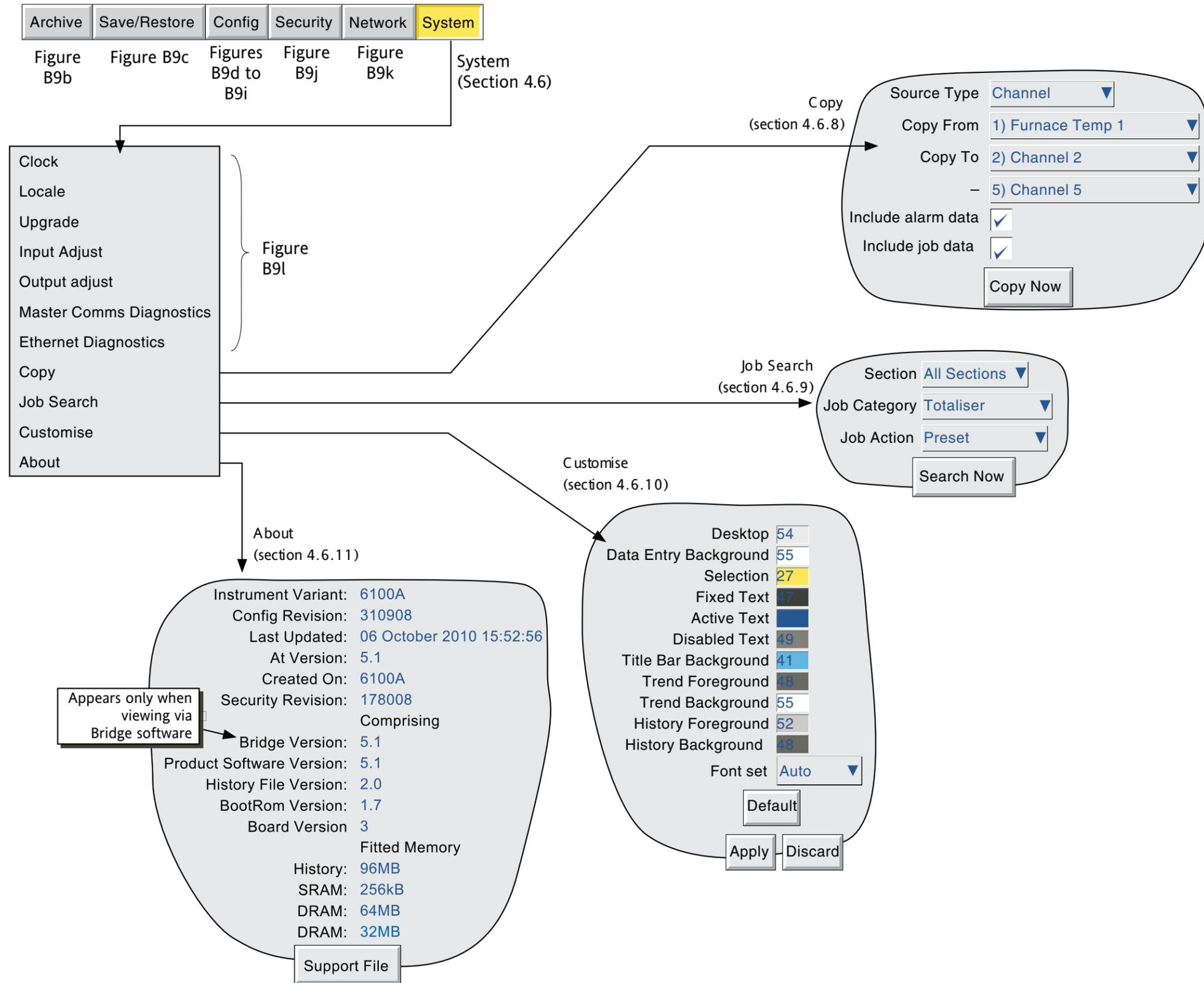
Figure B9m System key menu structure (sheet 2)
