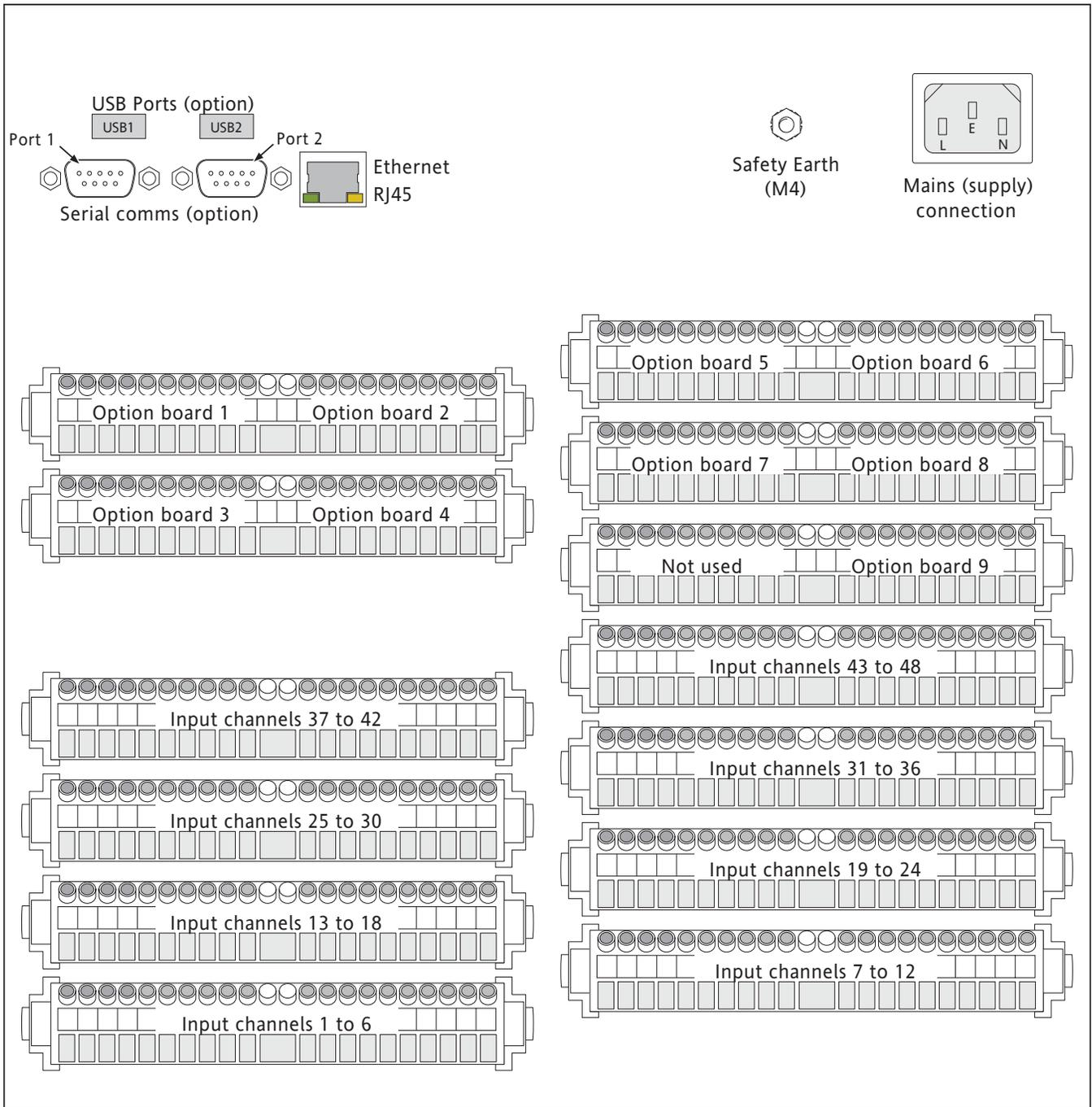
Figure 2.2.1b Connector locations - large frame units
