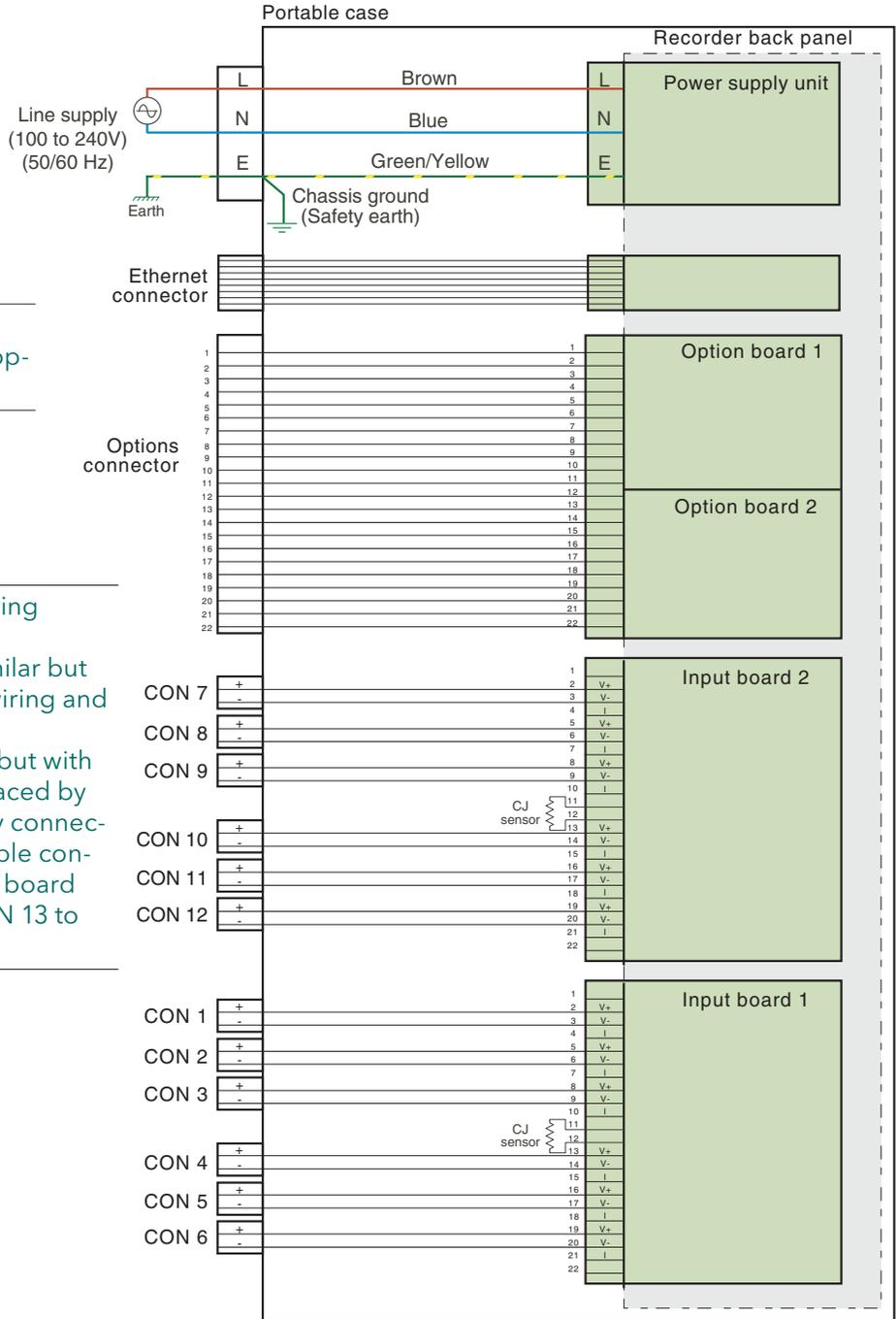
Figure 13.4.2c Internal wiring
