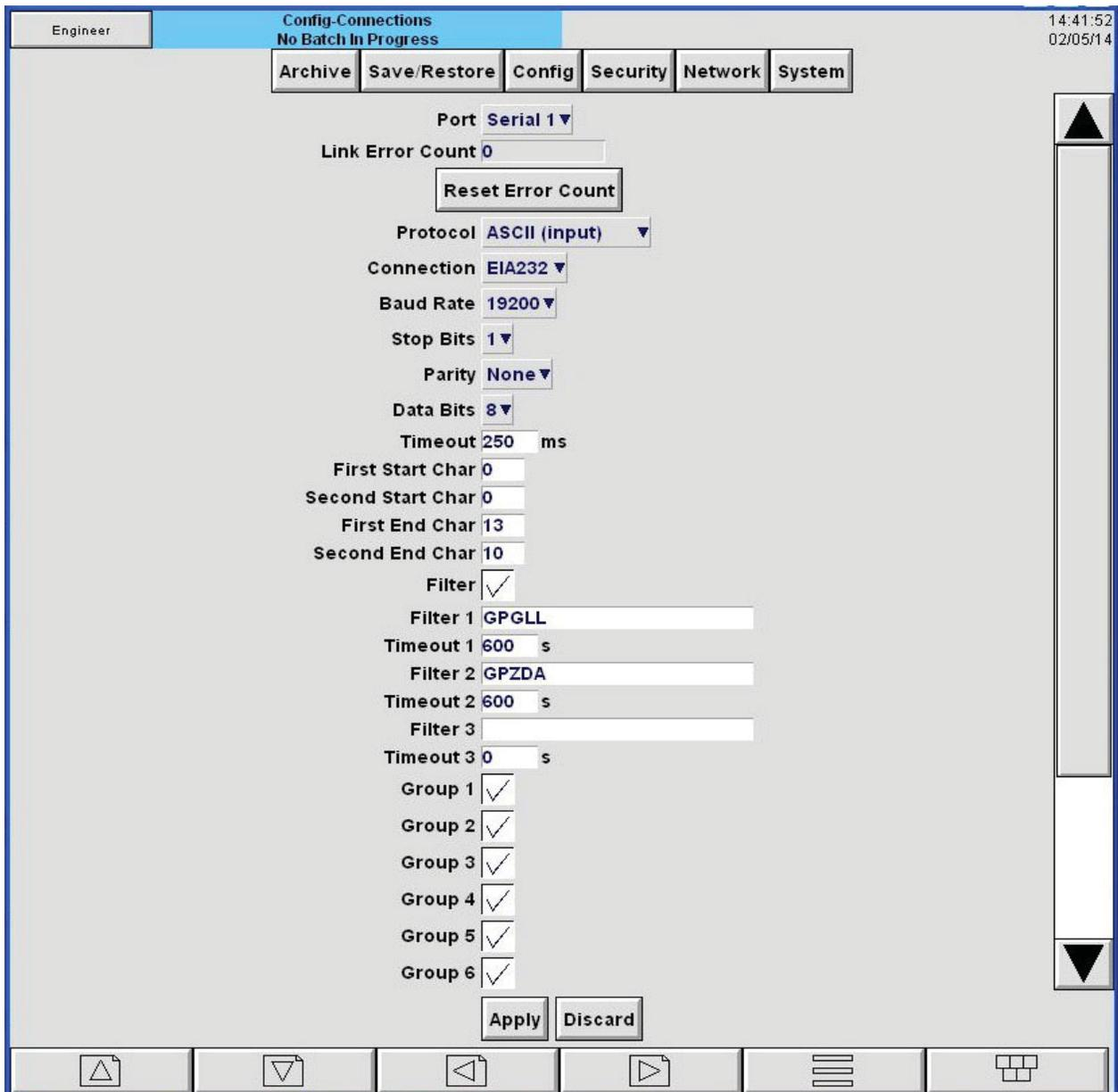
To enable the feature the 'Filter' parameter must be ticked. The filter parameters (1 to 3) will then appear. This is the default.
