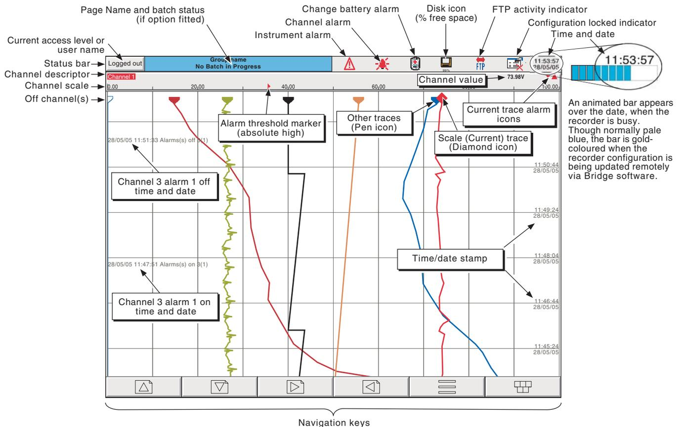
Figure 3 Trend display definitions (large frame unit)
