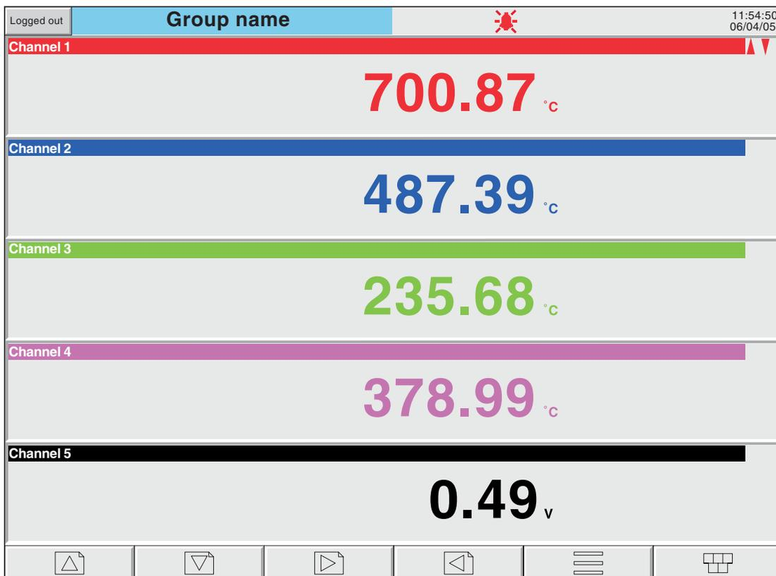
Figure 3.4.6a Numeric display mode (1 to 5 channels example)
