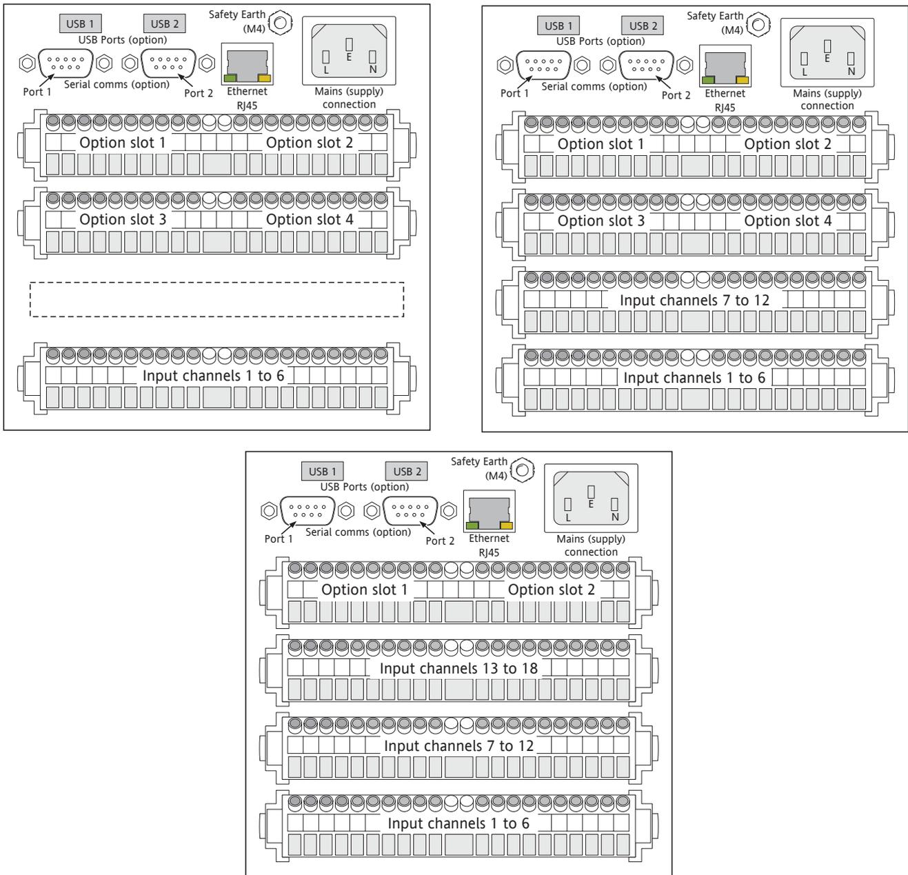
Figure 2.2.1a Connector locations - small frame units
