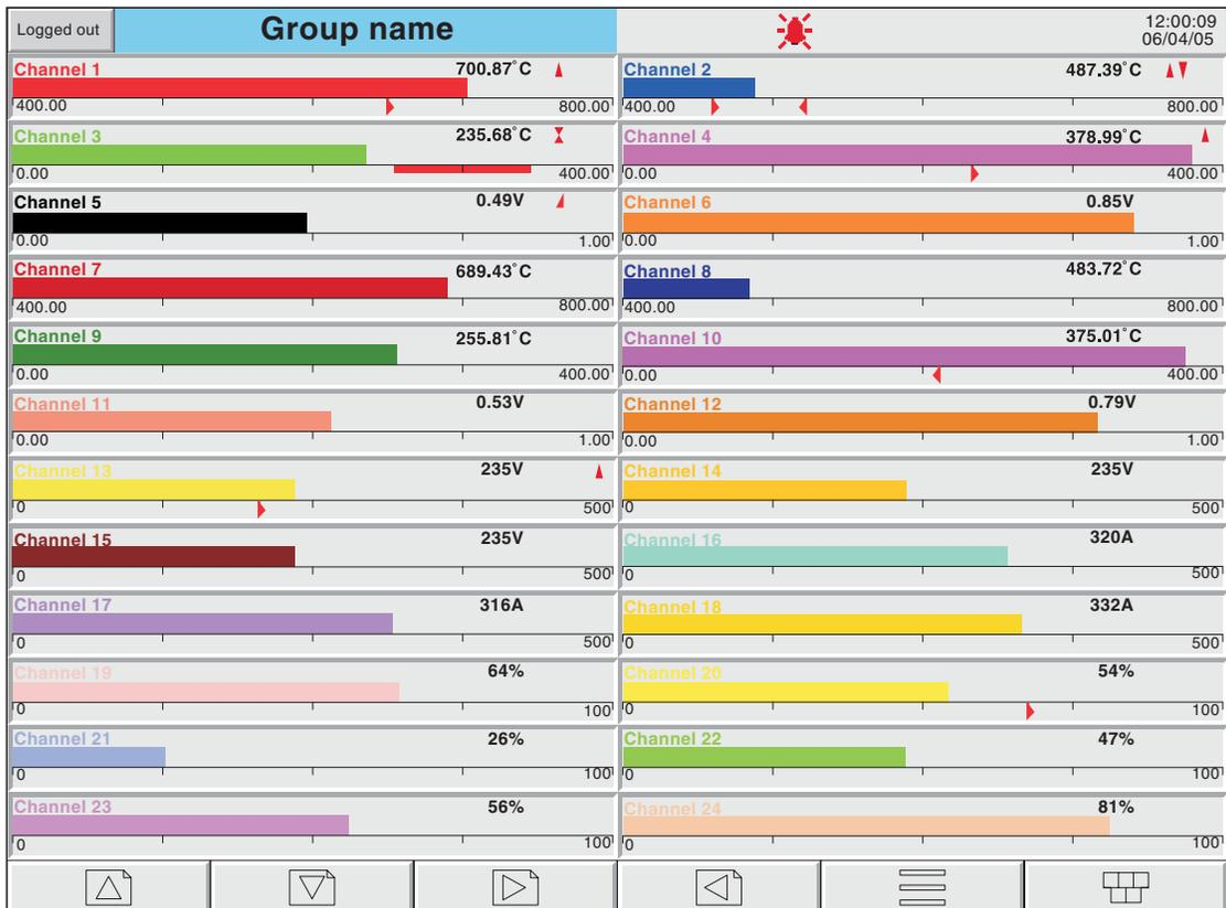
Figure 3.4.5b Horizontal bargraph display (dual column example)
