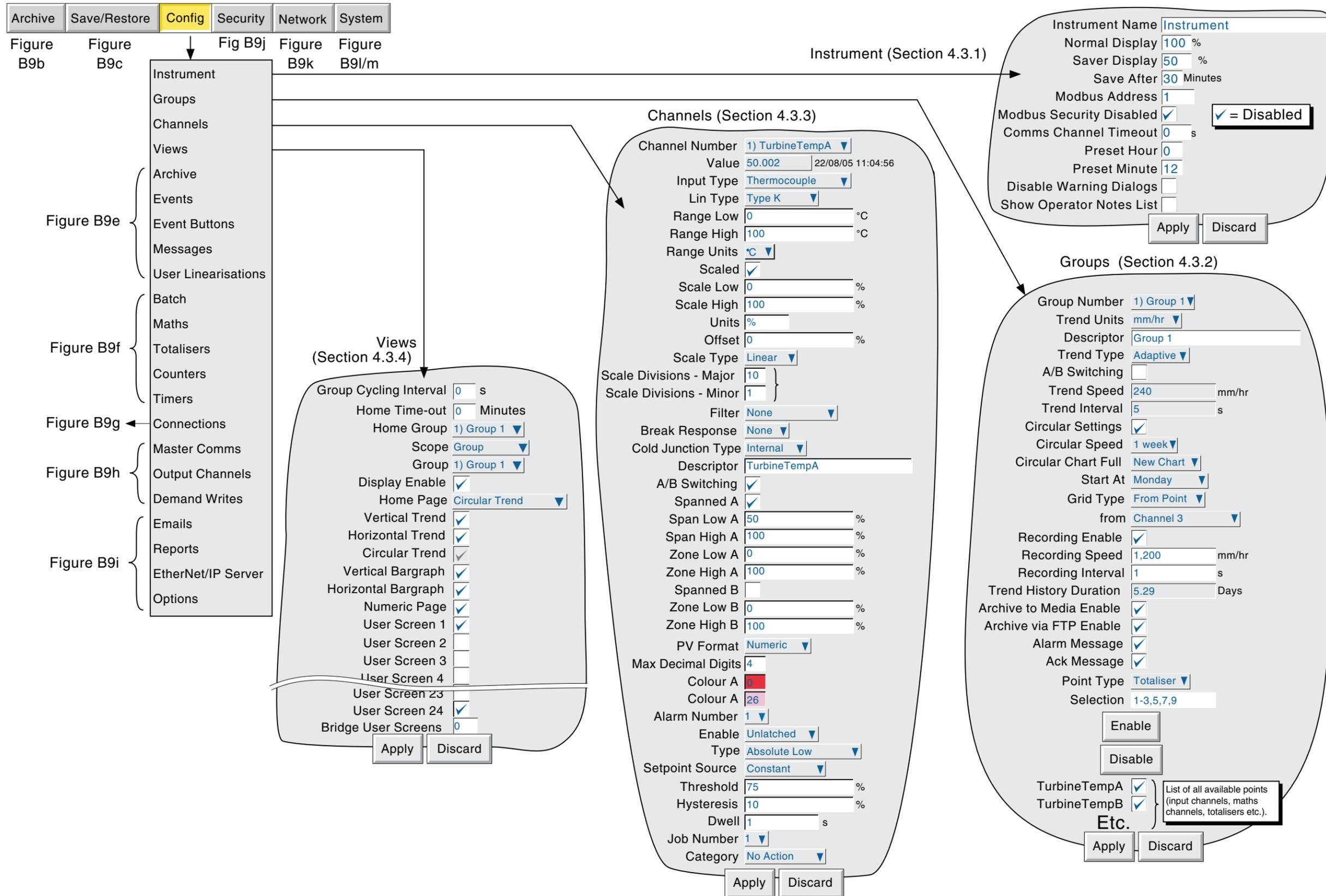
Figure B9d Config menu structure (sheet 1)
