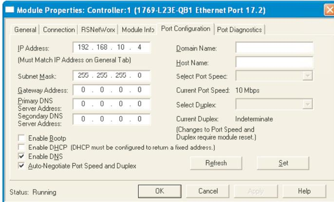
Figure 4.3.21i Module Properties
