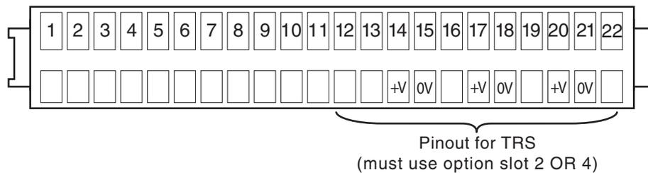
Figure 13.2 TRS pinout
