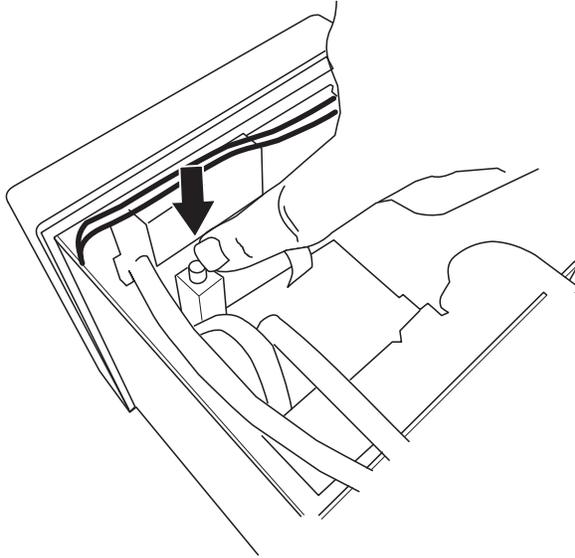
Fig 2.3a Flap release - small frame units
