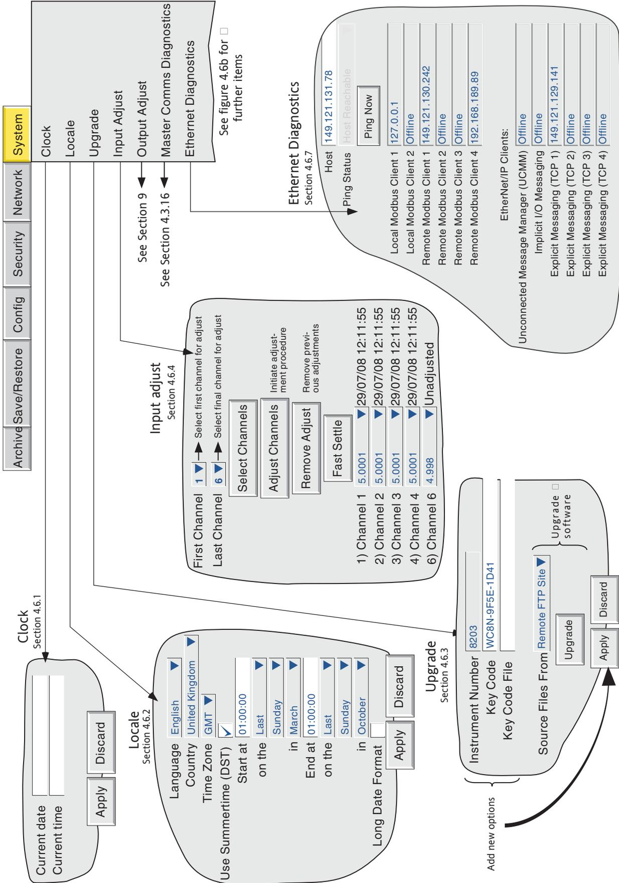
Figure 4.6a System configuration menu layout (sheet 1)
