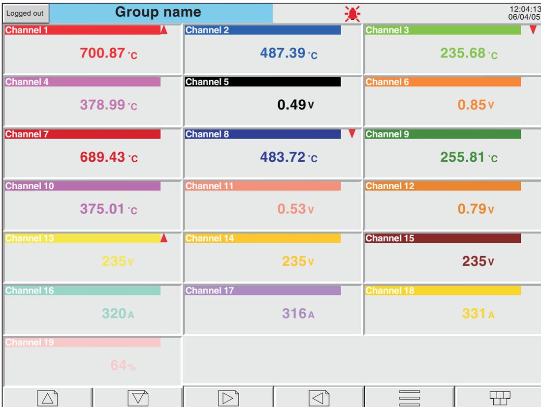
Figure 3.4.6c Numeric display mode example (19 channels)
