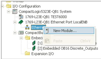
Figure 4.3.21l Right click on the EtherNet symbol
