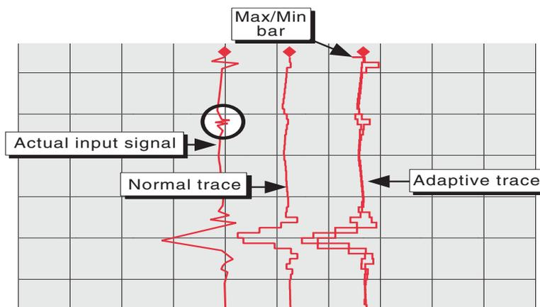
Figure 4.3.2b Adaptive recording compared with Normal tracing
