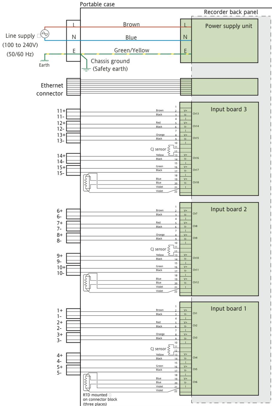
Figure 13.6.2c Internal wiring
