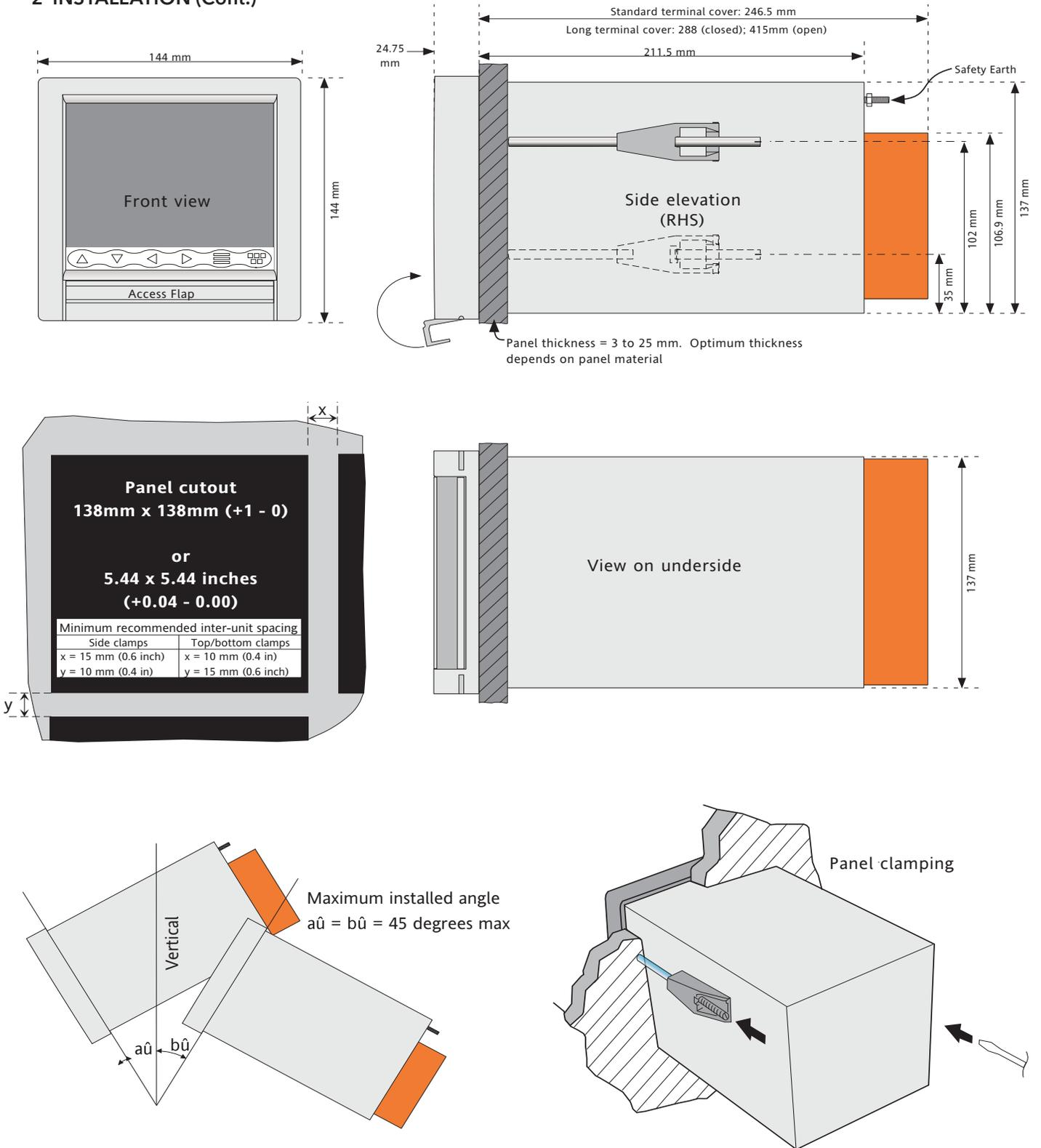
Figure 2.1a Mechanical installation details - small frame unit
