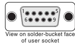
View on solder-bucket face of user socket
