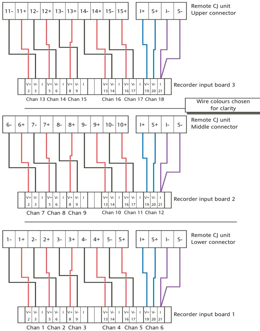
Figure 14.3.2c Wiring details
