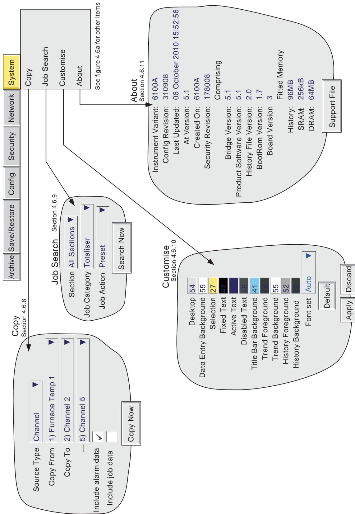
Figure 4.6b System configuration menu layout (sheet 2)
