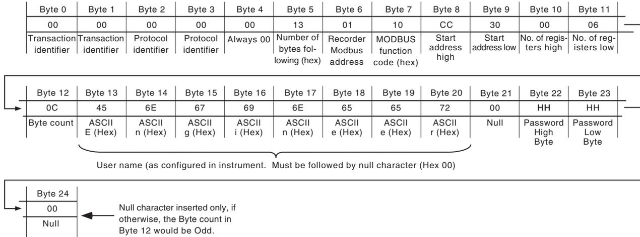
Figure 8.2.4a Login request via Ethernet (Modbus TCP)
