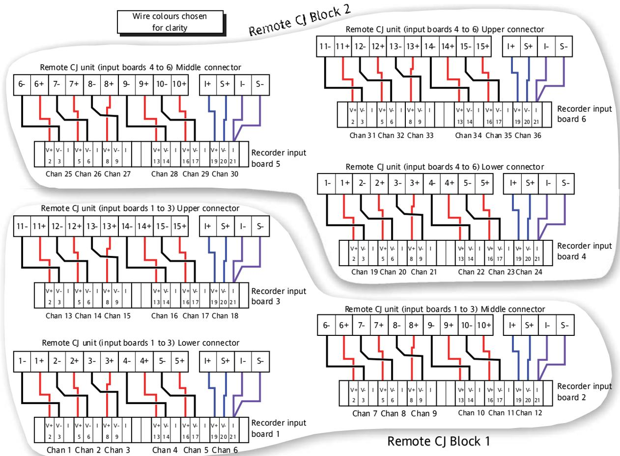
Figure 14.2.2c Wiring details
